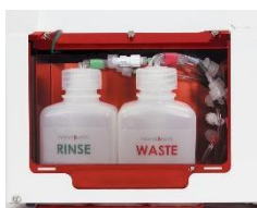
Fast access to 125 mL fluid containers
